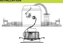
Socket adapter removes from module, allowing installation to be guick and easy. Simply screw in the adapter and plug in the module. Turning off the entire module is not required.
