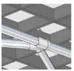
When installing into a hard-lid ceiling, secure the assembly with mounting screws using the holes at the connector points.
