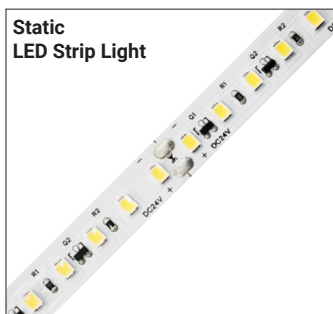
Series-LB1000-LR | 295lm/ft - 3.1W/ft Indoor Strip Light Width / 0.39"/10mm 37 LEDs/FT
