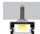
Profile with surface mounting clip
