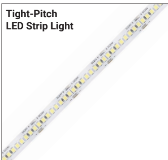
Series-LB1000-ST | 235lm/ft - 1.9W/ft Indoor Strip Light Width / 0.39"/10mm 72 LEDs/FT 565lm/ft - 4.6W/ft 875lm/ft - 7.2W/ft 1120lm/ft - 9.0W/ft 1400lm/ft - 11.1W/ft
