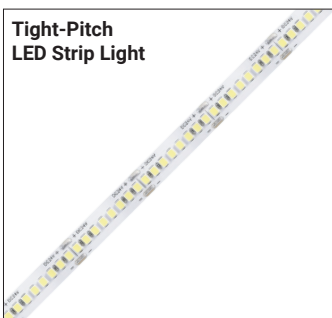
Tight-Pitch LED Strip Light Series-LB1000-ST | 235lm/ft - 1.9W/ft Indoor Strip Light | 565lm/ft - 4.6W/ft Width / 0.39"/10mm | 875lm/ft - 7.2W/ft 72 LEDs/FT | 1120lm/ft - 9.0W/ft 1400lm/ft - 11.1W/ft
