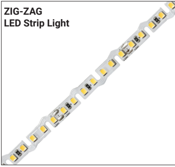
Series-LB1000-ZZ-ST | 455lm/ft -3.6W/ft Indoor Strip Light Width / 0.39"/10mm 43 LEDs/FT
