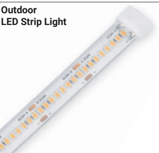
Series-LB1000-WL-ST | 215lm/ft - 1.9W/ft Outdoor Strip Light Width / 0.53" / 13mm 72 LEDs/FT 565lm/ft - 4.6W/ft
