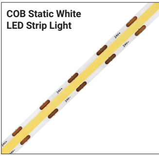
Series-LB3000-ST | 325lm/ft - 3W/ft Indoor Strip Light Width / 0.3"/8mm 146 LEDs/FT
