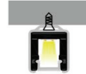
Profile with surface mounting clip
