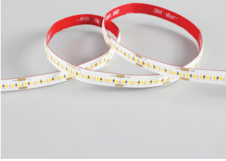
Series-LB1000V-ST | 890lm/ft-6.6W/ft Indoor Strip Light Width / 0.39" / 10mm 73 LEDs/FT
