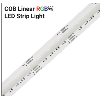
Series-LB3000-RGBW | 255lm/ft - 6.1W/ft Indoor Strip Light Width / 0.47" / 12mm 256 LEDs/FT
