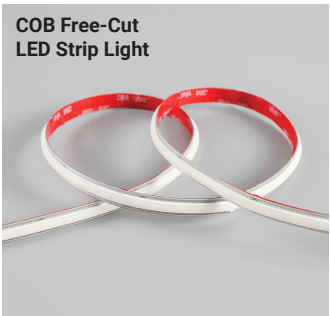
Series-LB3000-FC-ST | 550lm/ft - 4.6W/ft Indoor Strip Light Width / 0.39" / 10mm 98 LEDs/FT
