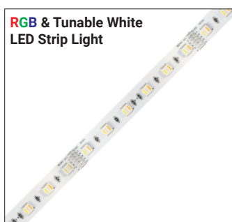
Series-LB4000-RGBTWH | 220lm/ft - 3.7W/ft Indoor Strip Light Width / 0.47"/12mm 18 LEDs/FT
