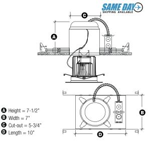
TO BE USED WITH 900 LUMEN LED MODULE LIGHTING COMPONENT
