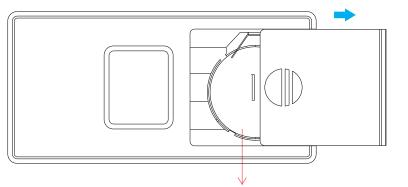
Note: Before the first use, please remove the protective film on the battery.
