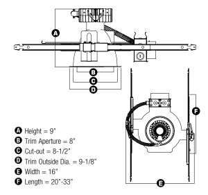
**DESCRIPTION** - 8" LED dedicated Architectural New Construction Downlight with integral LED heat management casting and driver (installed on junction box). Available in 800 lumens, 1100 lumens, 1500 lumens and 2000 lumens. Lighting is smooth and comfortable while using 50% less energy than the common 26W & 32W CFL downlight. Plus the eco-friendly MAXILUME LED system features 70% lumen maintenance at 50,000hrs of life, with California Title-24 (compliances pending).
