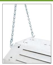
**CH** - Heavy Duty Chain comes with S hooks that attach directly to predrilled holes in High Bay fixture. Comes in a standard 6' length. Chain secures fixture to structure and installs easily.
