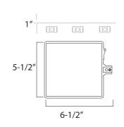
Finish: AWH-Architectural White ABK-Architectural Black Single Circuit Track Limiter live-end feed with circuit breaker
