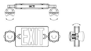
This product is an ideal for when both an exit sign and an emergency light are required. Its design makes it suitable for use above doors. Field selectable switch enables the sign to change from red to green and vice-versa.
