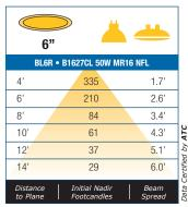
BEAM DIA, MEASURED AT 50% OF NADIR F.C.
