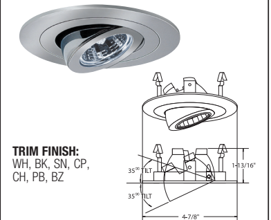
B1412CH FULLY ADJUSTABLE (35° TILT, 359° ROT.)
