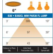
BEAM DIA. MEASURED AT 50% OF NADIR F.C.
