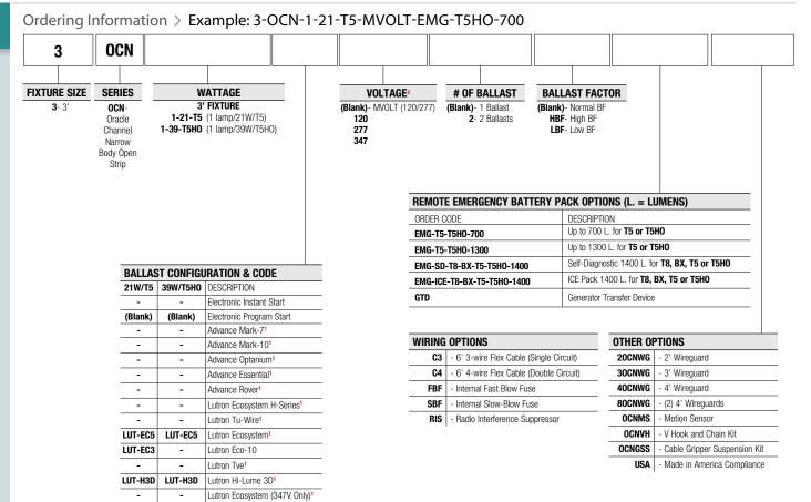
1- Voltage must be specified for dimming ballast.
