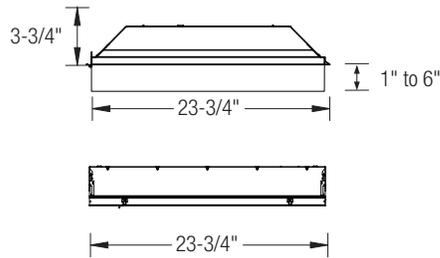
The CUBE-LED is a high-quality yet economical troffer luminaire powered by LED lighting technology, which offers the highest return on initial investment over the lifetime of the fixture. An excellent, highly efficient fixture, ideal for office spaces, schools, hospitals, and many other indoor applications. Compatible with most industry standard T-bar grids.
