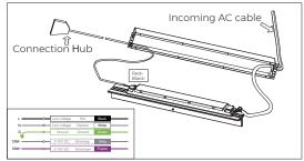
3. Connect the incoming AC wiring to the power supply according to the figure in the bottom left hand corner, and connect the connection hub cables to the DC output at the other end of power supply driver.
