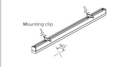
6. Before arrangement, rotate the mounting clips to the angle perpendicular to the light fixture.
