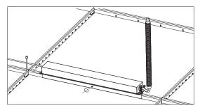
5. Fix the Junction box module assembled above, on to the T-bar keel and lock it in with screws.
