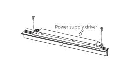
2. Use the screws to lock the power supply driver on to the junction box bracket.
