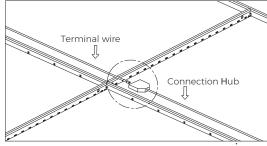
8. Insert the terminal wire from the fixture to the connection hub at the top of the ceiling. Cover the ceiling tile. After installation is complete, test light fixture to make sure it is working properly.
