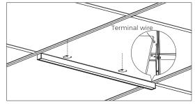
7. Open up ceiling tile, and put terminal wire from light fixture to top of ceiling. Mount the light fixture to the drop ceiling, by holding it against the T-bar, and turning the mounting clips counter clockwise to lock them on to the T-bar and securing it in place.
