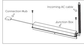
4. Lock the junction box using screws, and cover the incoming AC power line with protective metal tubing.
