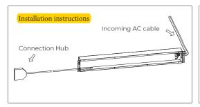
Use clamp to remove the metal cover of the junction box, and put the wiring for the connection Hub, and AC cables through the corresponding holes at each end of the junction box.
