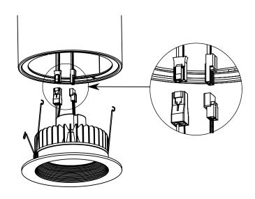
Squeeze the torsion springs and insert them into the slot bracket. Pushup the recessed downlight.
