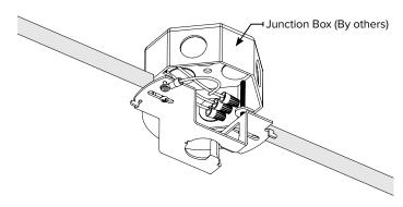
**3.** Insert ball joint through opening on universal mounting bracket and then align the groove on the ball joint with the tab on the universal mounting bracket..
