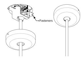
Screw threaded nut to threaded pendant stem, and then feed it through the hole and screw the second threaded nut inside the can.
