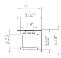
\*Brackets are mounted to a 4S junction box with a double gang plaster ring.
