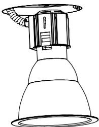
Gut out existing reflector and wiring from mounting frame and j-box respectively
