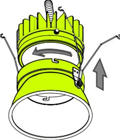
Push up the reflector then rotate it counter clockwise to secure the twist screws into reflector slots. Tighten both twist screws.
