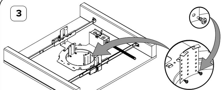
Screw in **MFG-BK-HHJ6-8-10-L** bracket into existing mounting frame.
