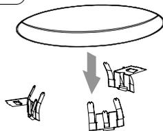
If needed remove any existing friction blades clips from the mounting frame.
