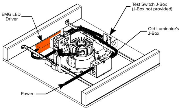
Lay down the EMG driver in the drywall ceiling..
