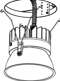
Insert the flange trim by squeezing v-spring into the bracket slot
