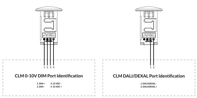
$NOTE: DEXAL\ is\ a\ DALI\ driver\ with\ self-powered\ DALI\ link.\ See\ Installation\ Instructions\ for\ additional\ wiring\ methods.$
